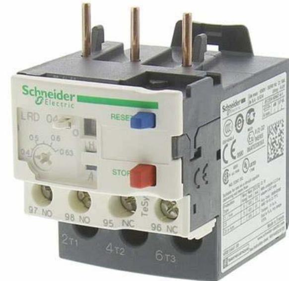
An **overload** relay is made up of a heater paired with normally-closed **contacts** that open once the heater gets too hot. The **overload contacts** are connected in series and located between the **contactor** and the motor itself to prevent the motor from restarting once the **overload** trips
